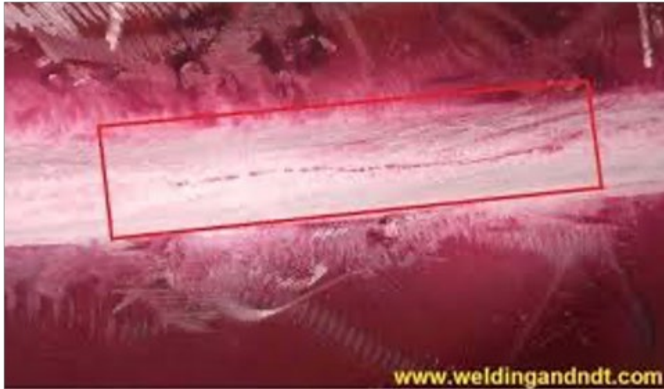
Figure 1. Example of dye penetrant test highlighting crack in test piece
