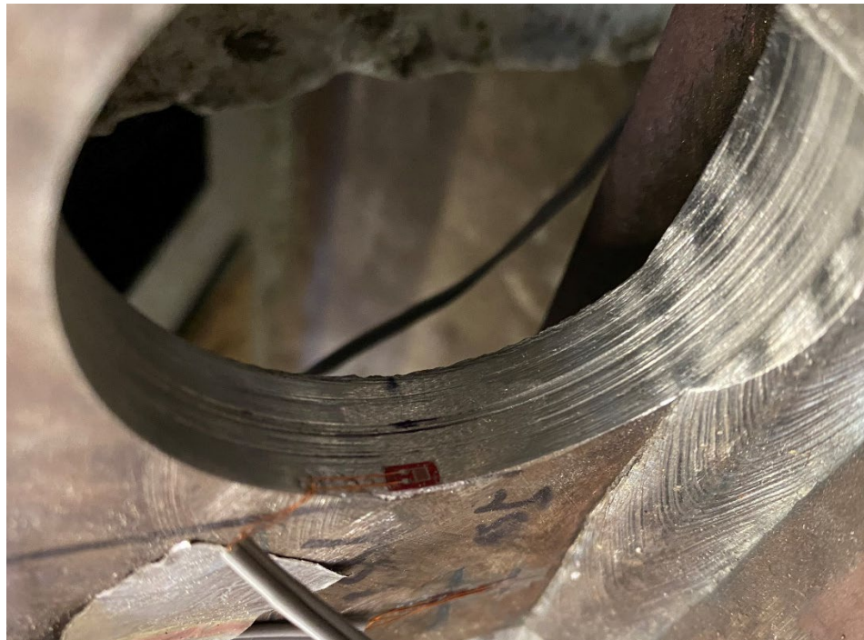
Figure 33. Edge of east CAH with edge gage installed for specimen SAW-12-25-4-2-N.
