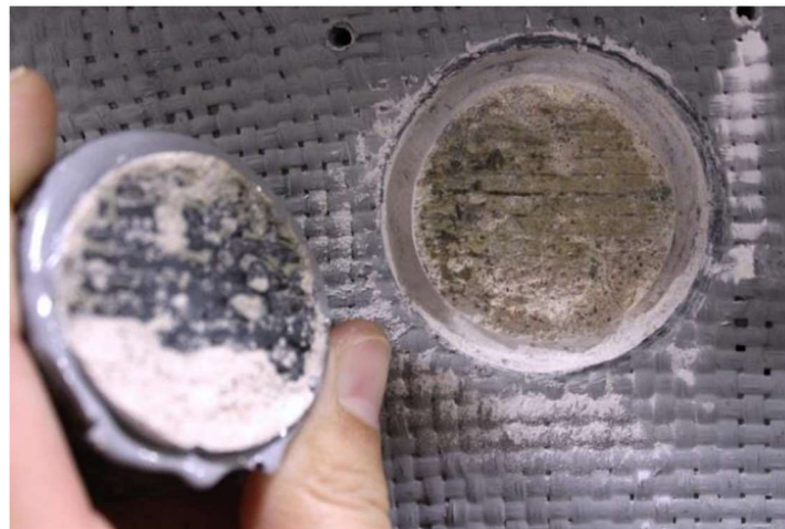
Figure 17. Adhesive failure mode observed on pull-off test.
