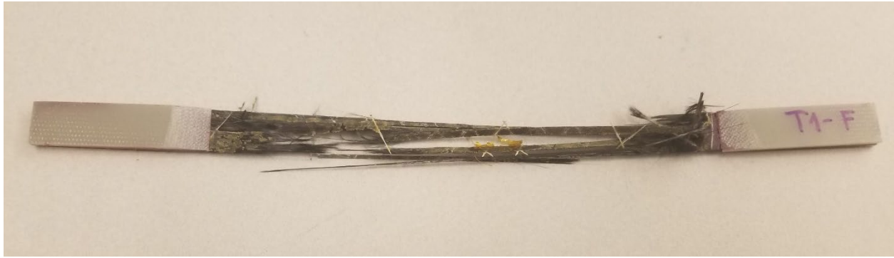
Figure 105. Typical failure mode of tensile test coupons.
