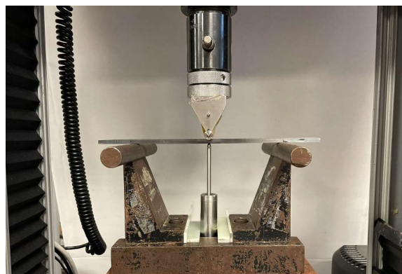
Figure 74. Three-point bending test setup.
