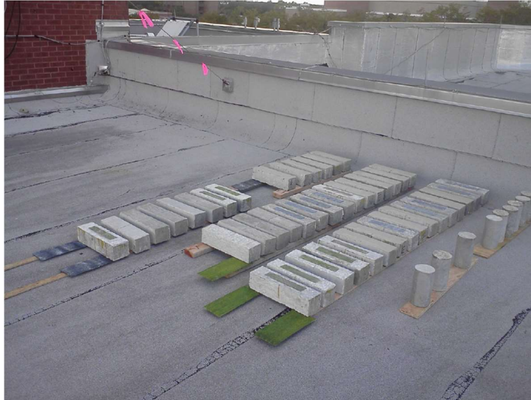
Figure 6. Field conditioning of concrete beam specimens and cylinders.
