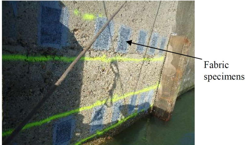
Figure 7. Bonded CFRP composite on a quay wall in the marine environment.
