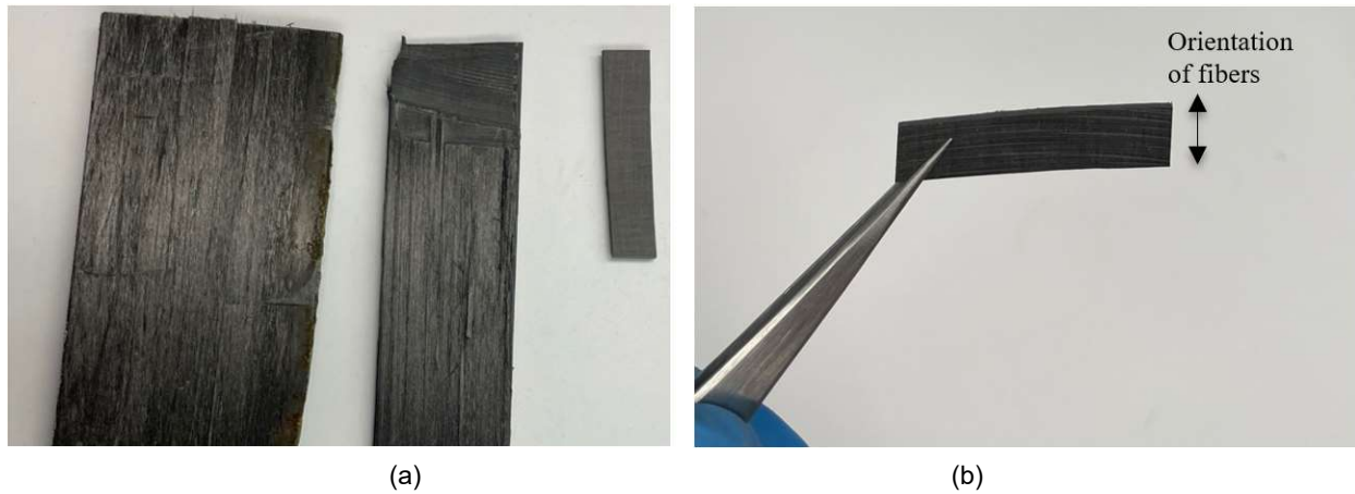
Figure 68. Preparation of DMA test specimen using the CFRP composite samples collected from the field: (a) loose fibers were sanded to make the surface even, and (b) final look of the sample ready for DMA testing.
