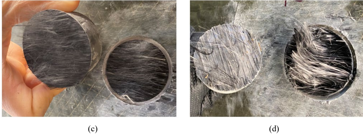
Figure 107. Two failure modes observed: (a) mode B on G1-U1, (b) mode E on G23-B1, (c) mode B on G4-UD1, and (d) mode B on G4-UD2.
