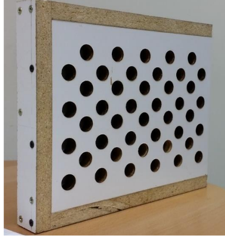
Figure 5. The symmetrical circular pattern for IR camera calibration.
