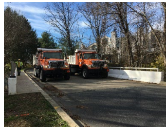
Figure 4: Loading position of trucks on DE 1-213 bridge
