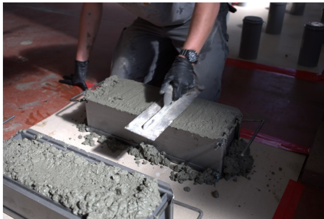
Figure 42. Finishing concrete within a 6 in. x 6 in. x 20 in. beam mold.
