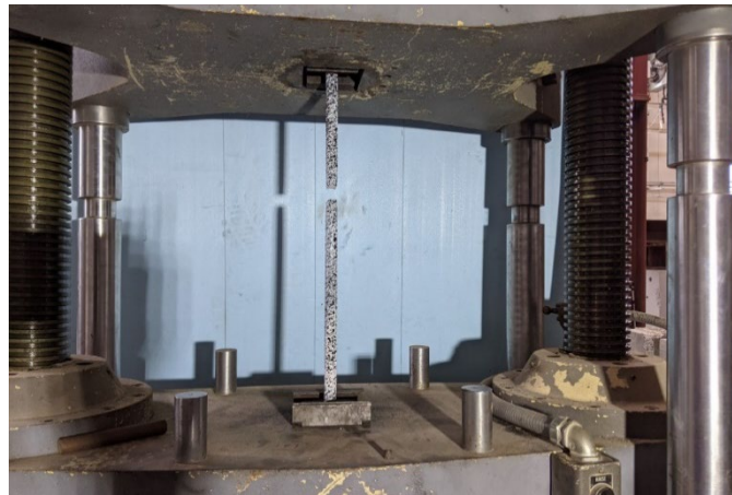
Figure 47. Ruptured rebar tensile test specimen.
