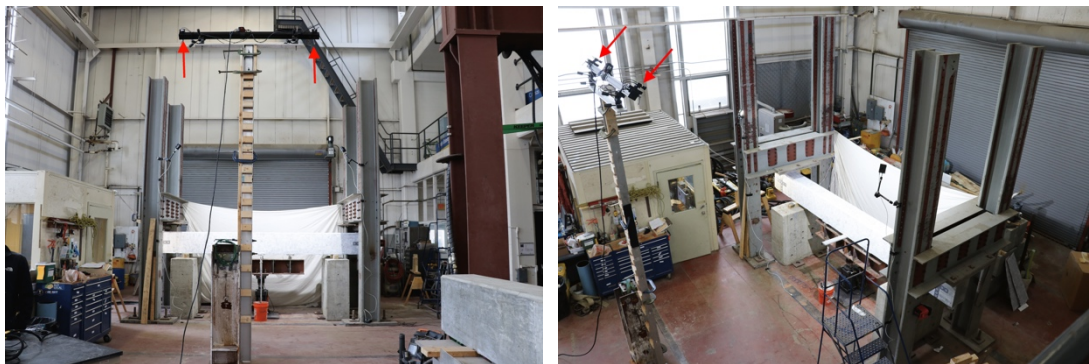
Figure 36. Photographs of the DIC system test (red arrows showing DIC cameras): (a) DIC system placed on top of the aluminum column; (b) test setup with the DIC system (red arrows showing DIC cameras).
