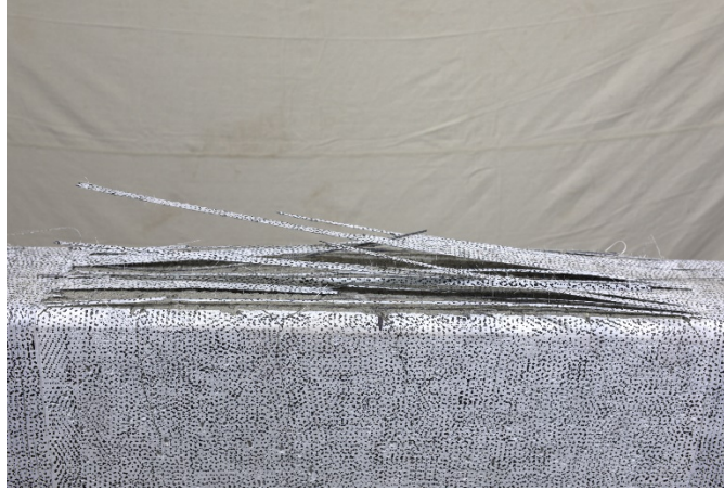
Figure 71. Rupture of the longitudinal CFRP within the constant moment region of 1L1U-8.
