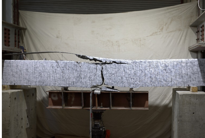
Figure 73. IC debonding failure of 2L0U. Girder was taken to concrete crushing post-debonding failure to investigate its residual strength.
