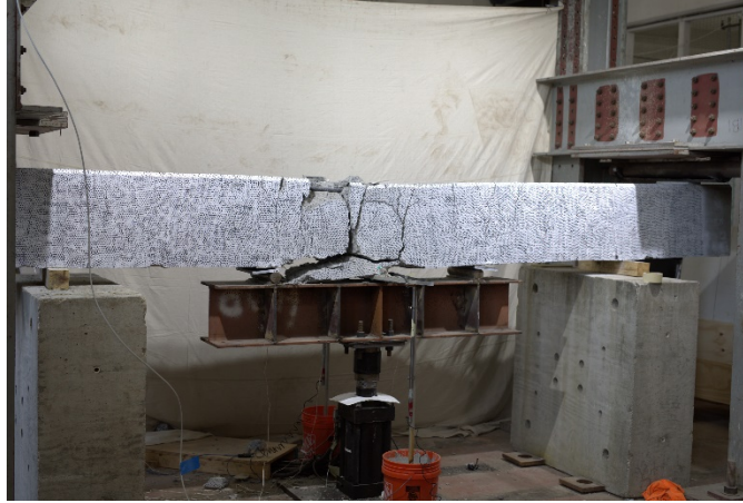
Figure 69. Concrete crushing failure of 0L0U
