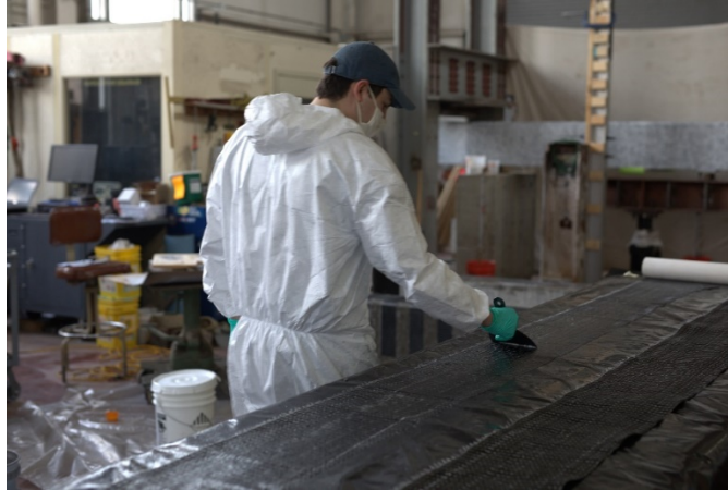
Figure 29. Spreading epoxy on the dry fibers using a putty knife within the epoxy bath.
