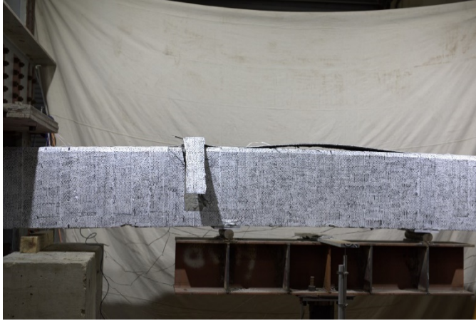
Figure 75. Complete U-Wrap debonding failure of 2L2U-8.
