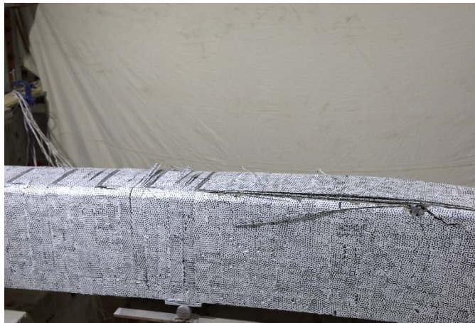
Figure 74. U-Wrap rupture failure of 2L1U-8.
