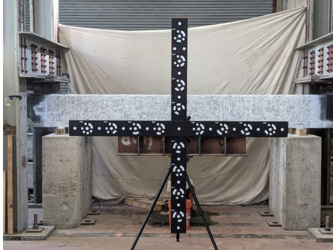
Figure 37. Calibration cross used for the DIC system.
