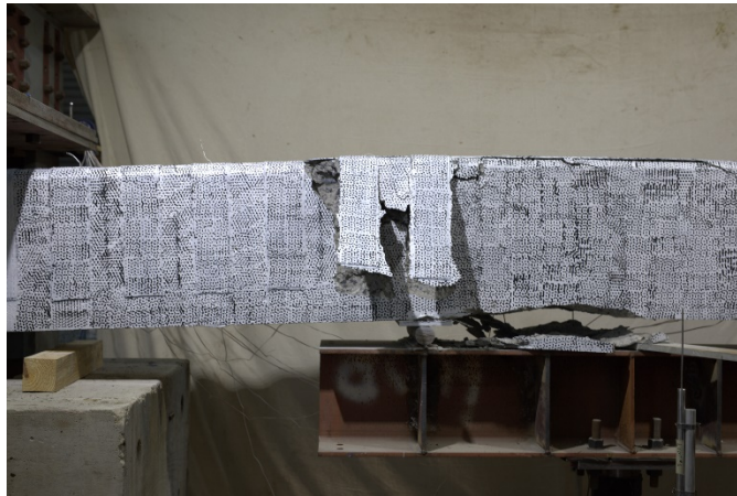
Figure 80. Concrete crushing failure of 3L3U-8. Secondary failure mode of complete U-Wrap debonding was observed.
