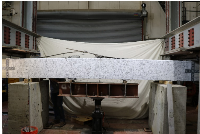
Figure 70. IC debonding failure of 1L0U
