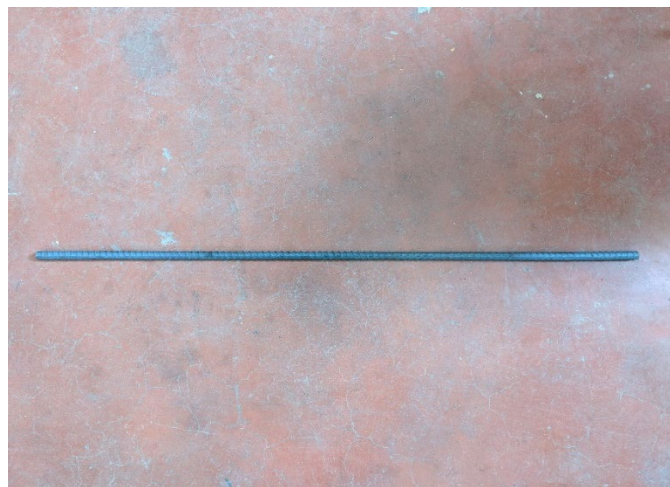
Figure 46. Typical 4-ft section of #6 rebar used for tensile tests.
