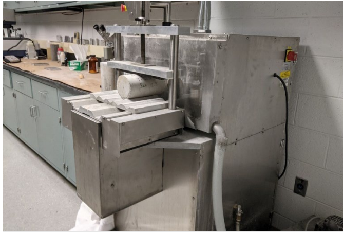
Figure 43. Grinding the top surface of the concrete cylinder.
