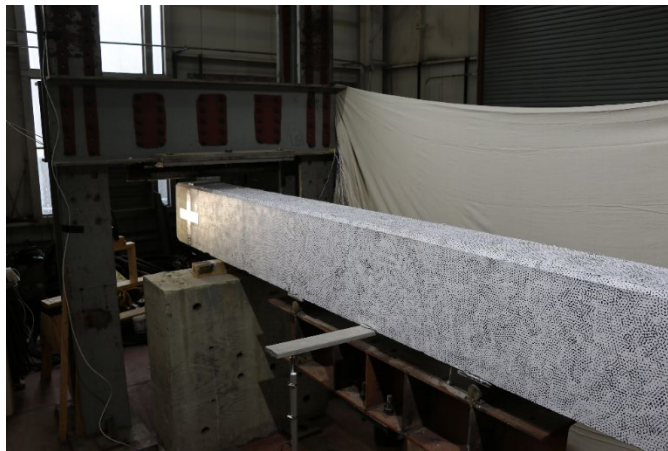
Figure 38. Speckled pattern applied to the vertical and tension faces of the girder.
