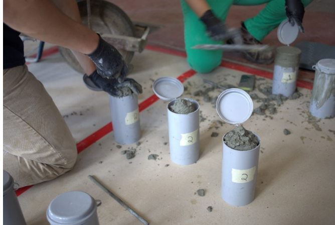
Figure 41. Filling concrete into 4 in. x 8 in. cylinder molds.
