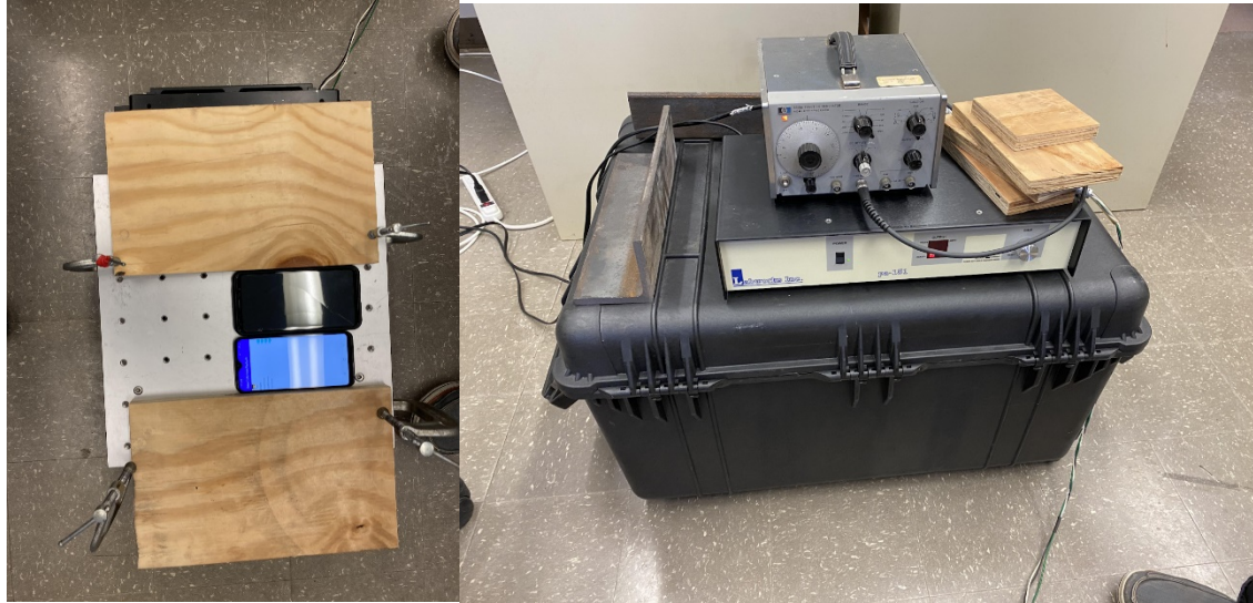
Figure 7. Experimental setup for testing the data collection API: (left) two smartphones attached to a shaking table, (right) signal generator for shaking table.
