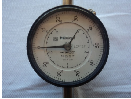
Figure 3.13. Mitutoyo dial gauge model 2424S-19, 5-cm (2-in.) travel, LC 0.00254 cm (0.001 in.).
