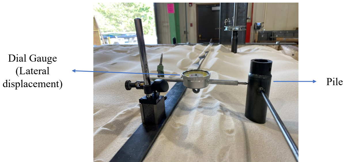
Figure 3.17. Data acquisition for lateral load tests.
