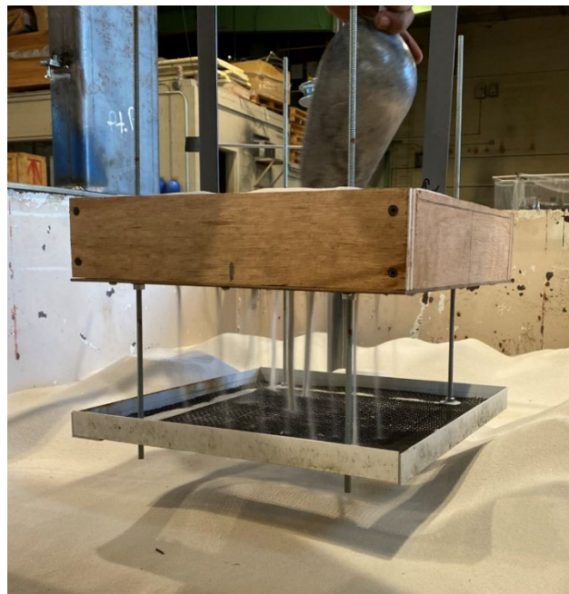
Figure 3.5. Pluviator including sieves used for preparing medium dense sand deposits ( D_r=45\%-55\% ).
