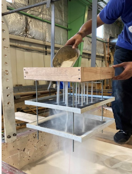
Figure 3.4. Pluviator including sieves used for preparing dense sand deposits ( D_r=75\%-85\% ).
