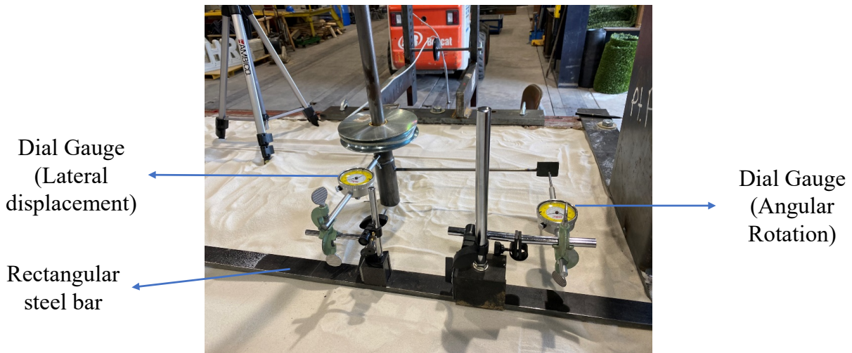
Figure 3.16. Data acquisition setup for torsional load tests.
