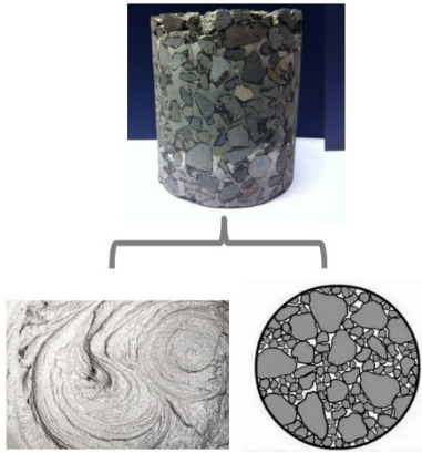
Figure 6. Appearance and composition of the SFCM.
